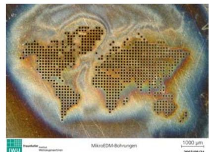
Micro bore array (bore dia.  $85\mu\text{m}$ , depth  $800\mu\text{m}$ , distance  $125\mu\text{m}$ , overall size  $5.5 \times 3.0\text{mm}$ , US-assisted)
