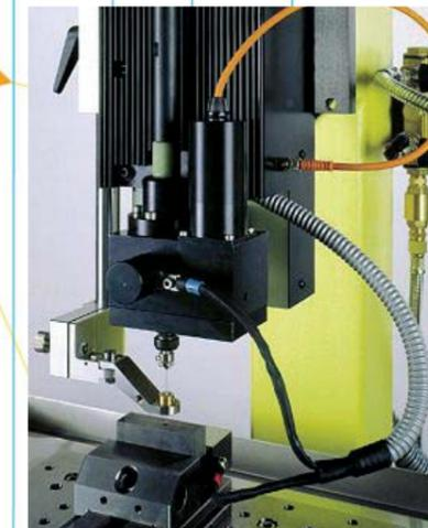
SX-RHP spindle with manual electrode re-feeding
