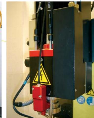
SX-A344 spindle with automatic electrode re-feeding
