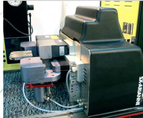
The SX-ARIANNE as "built-in" unit is mounted on the machine table. The status monitoring of the unit appears immediately on the SX-MMI command panel. In the event of operating requirements change or another machining operation the unit can be easily removed or mounted minimizing down time.
