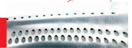
The SARIX  $\mu$ EDM technology distinguishes itself by high process reliability and repeatability. The SARIX production machine is generally used for hole sizes between 50 microns and 3 mm.
